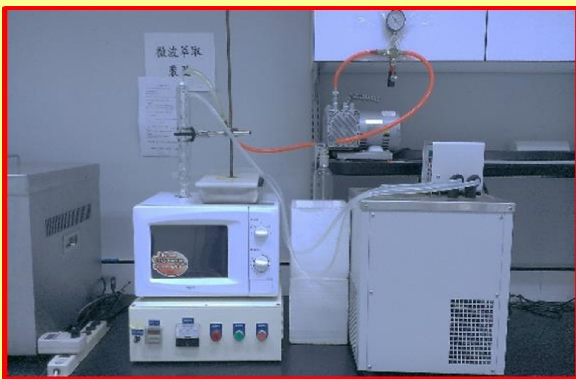
Fig. 1. Photograph of the microwave vacuum extraction system.
