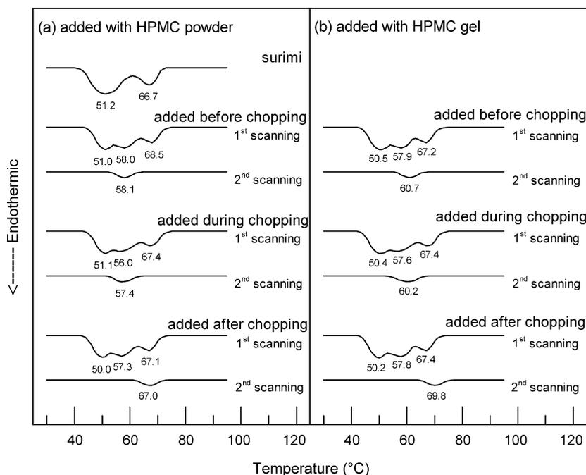
Fig. 5. DSC programs of reheated test in surimi with (a) HPMC powder and (b) HPMC gel solution added at various chopping stage.
