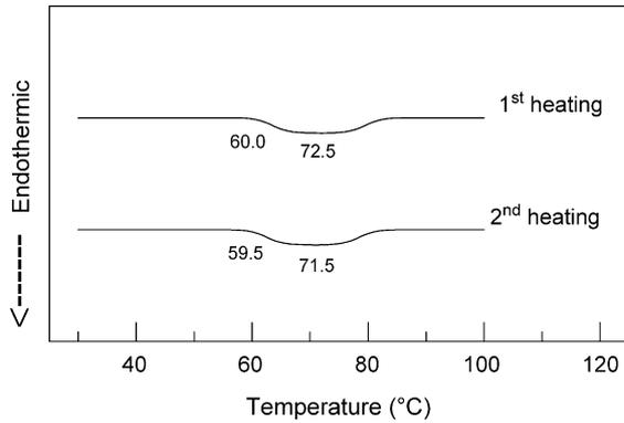
Fig. 2. DSC programs for rescanning test for a 20% HPMC gel solution.
