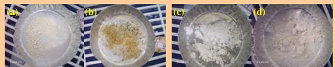
Fig. 6 Pictures of spray-dried powders stored at 25 °C with different RH three days, Blank: (a) 33% (b) 75% ; HPMC: (c) 33% (d) 75%
