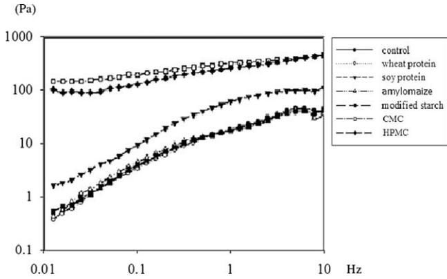
Fig. 1. The  $G'$  (storage modulus) values of different batters at 25 °C.
