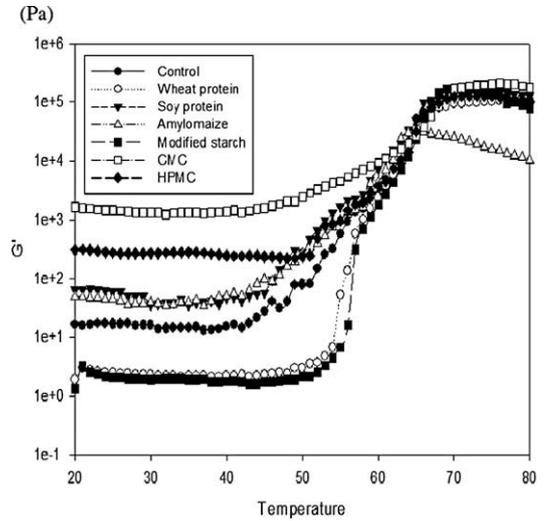
Fig. 4. Effect of temperature gradient on  $G'$  values for different batters.
