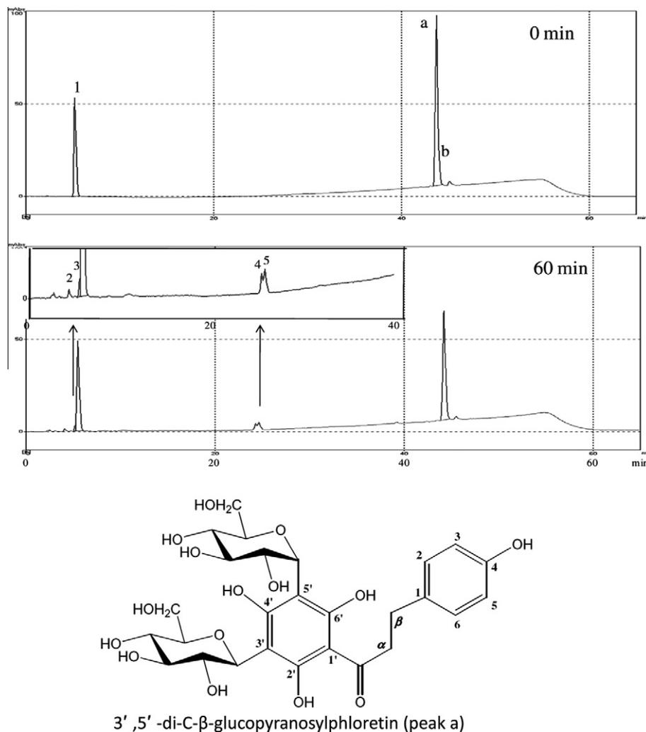
**Fig. 1.** HPLC analysis of the reaction solution after addition of ICW-V, tyrosine and tyrosinase for different duration. (a: 3',5'-di-C-β-glucopyranosylphloretin, b: unknown, 1: tyrosine, 2: DOPA, 3, 4, and 5: unknown).
